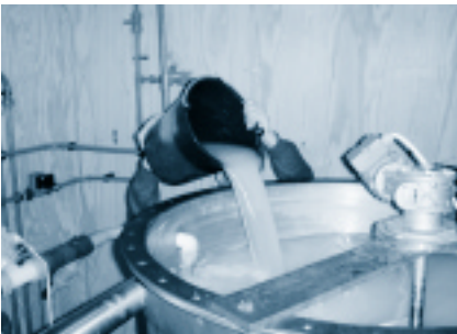
The ice slurry is being collected in 9 m 3 storage tanks.
