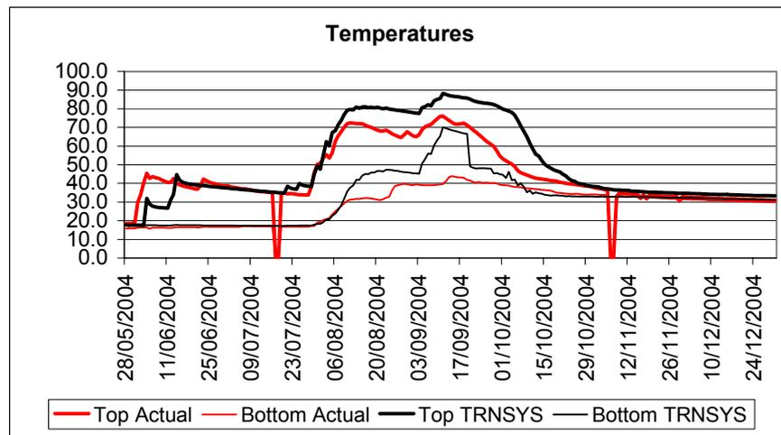
Fig. 2.41 Storage temperatures, combined
