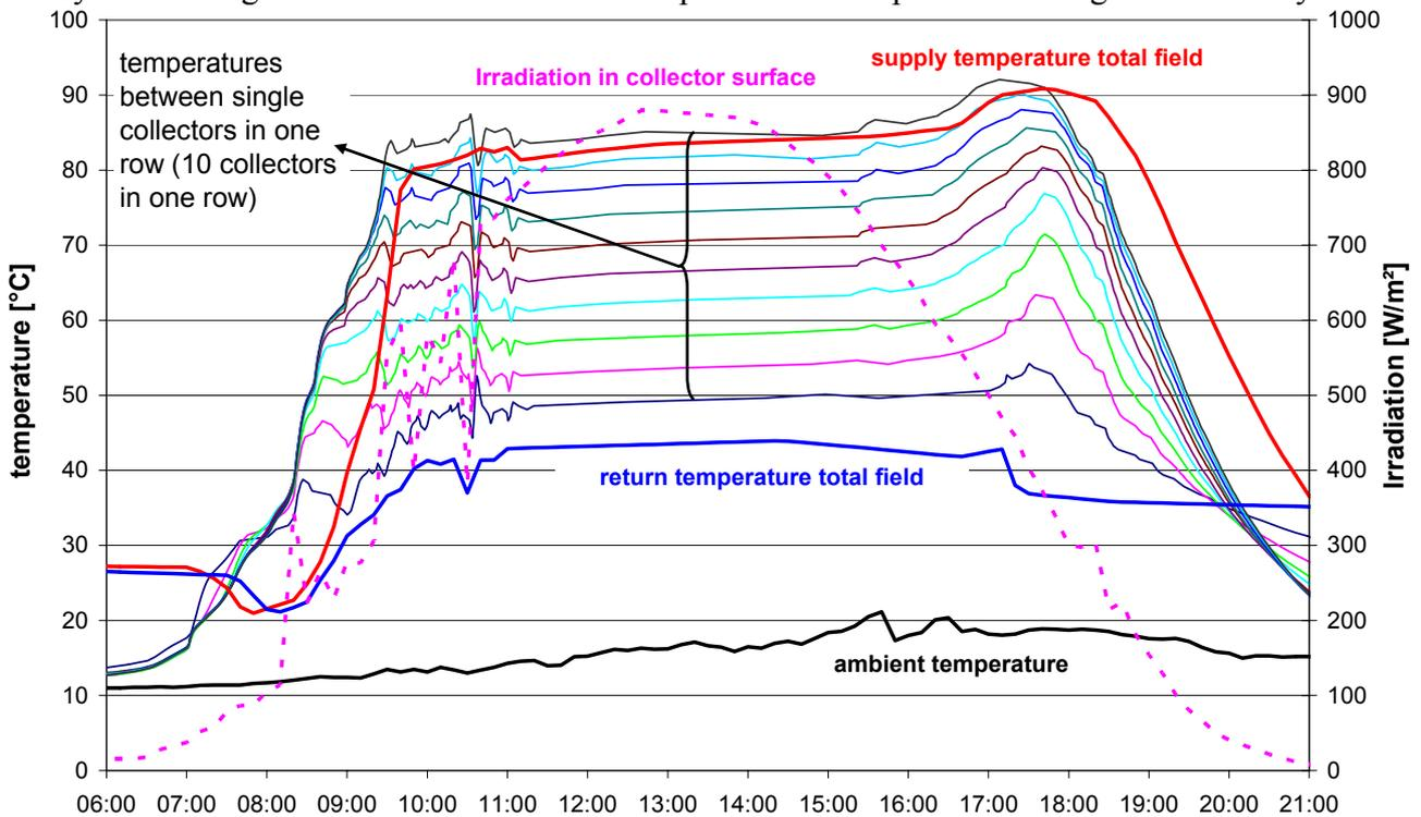
Fig. 2.23: Temperature development within the new Arcon field (09.05.2004)
