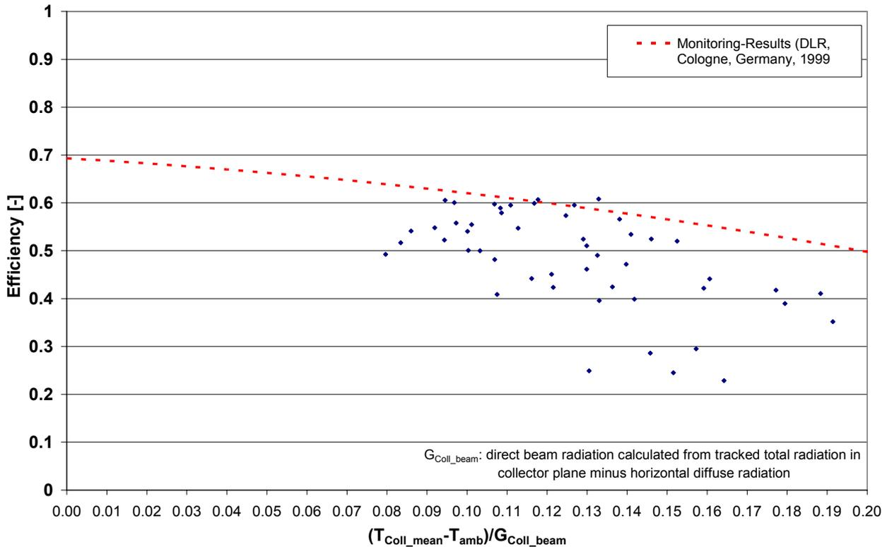
Fig. 2.27: Collector field efficiency IST field (parabolic troughs, 211 m<sup>2</sup>)
