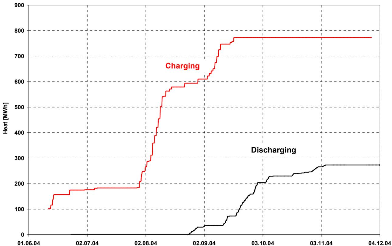
Fig. 2.28: Charging and discharging of the pit heat store
