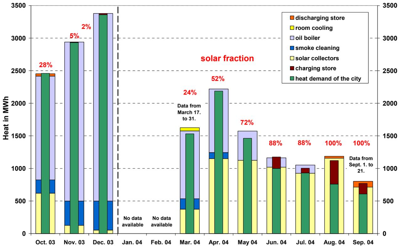
System heat from October 2003 to September 2004 according to heat meter data.
