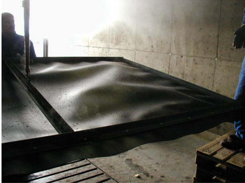
*Fig. 2.8. Expansion experiment. 2.5 mm HDPE. 70 °C.*
