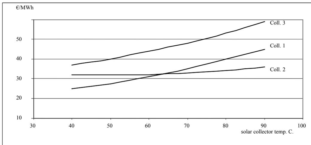
*Example of production prices/kWh for different solar collectors at different mean heat temperatures.*
