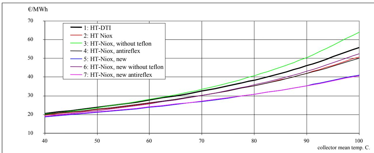
Fig. 2.3. Production price for heat for different collector combinations with Sunstrip absorbers.
