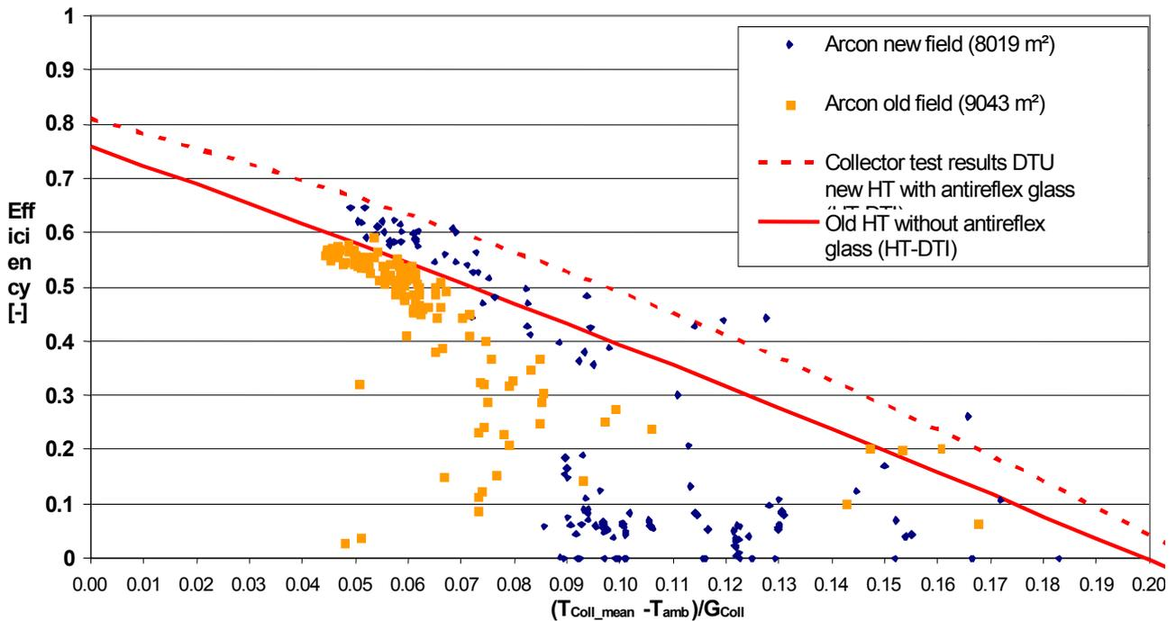
Collector field efficiency Arcon collector fields.
