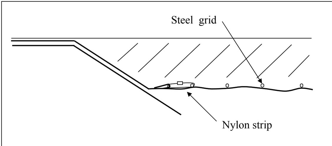
Fig. 2.9. Steel grid to counteract expansion.
