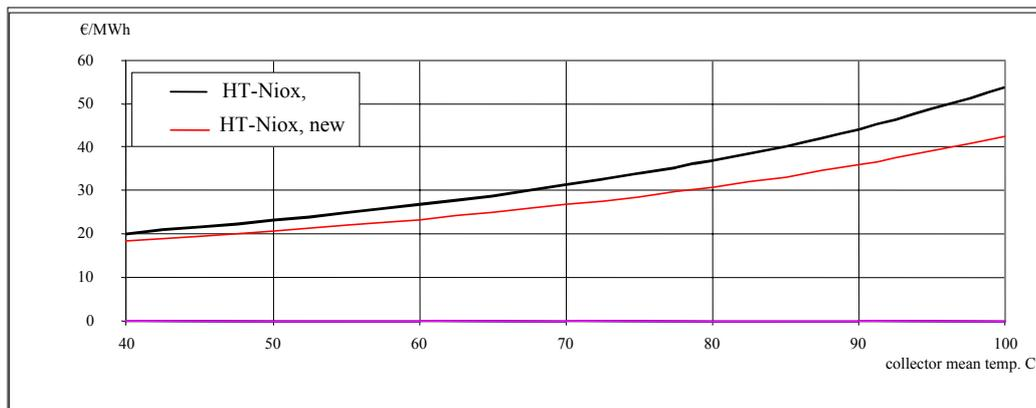
Fig. 2.6. Production prices (€/MWh) for the older and the new ARCON-HT collector
