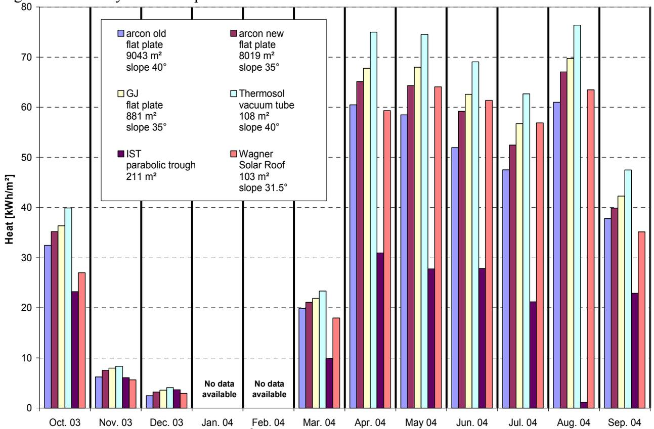
Fig. 2.20: Solar heat production per m<sup>2</sup> collector area.
