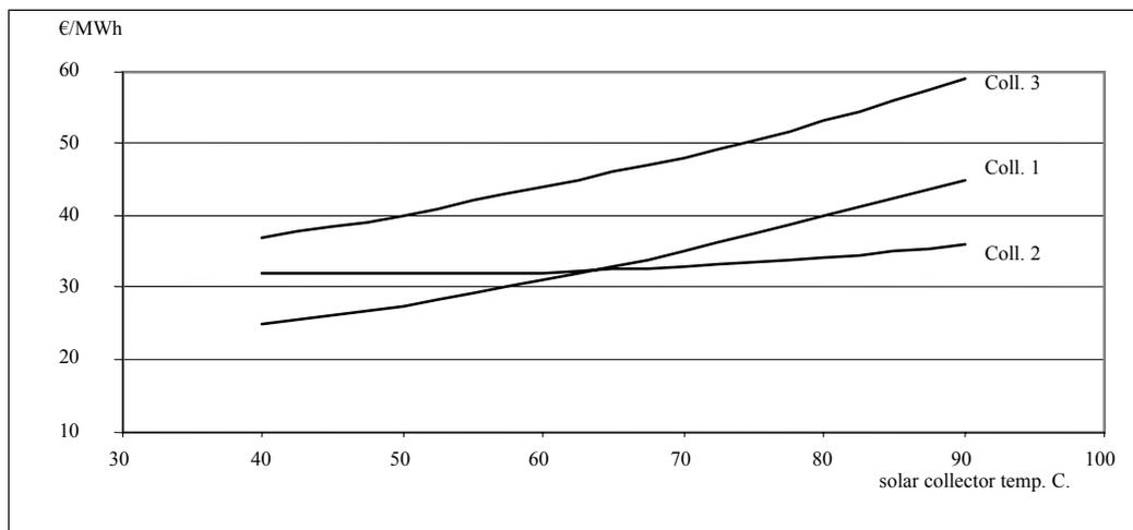
Fig. 2.2. production prices/MWh for different solar collectors at different mean heat temperatures.
