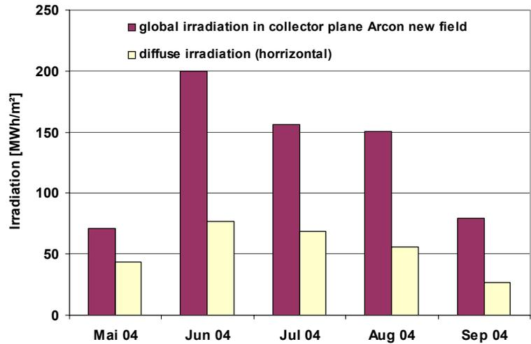
Fig. 2.21: Global and diffuse irradiation (global: tilted 35°, orientation south; diffuse: horizontal)
