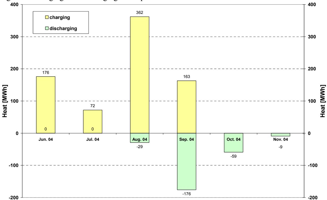
Fig. 2.29: Heat balance of the pit heat store from March to November 2004
