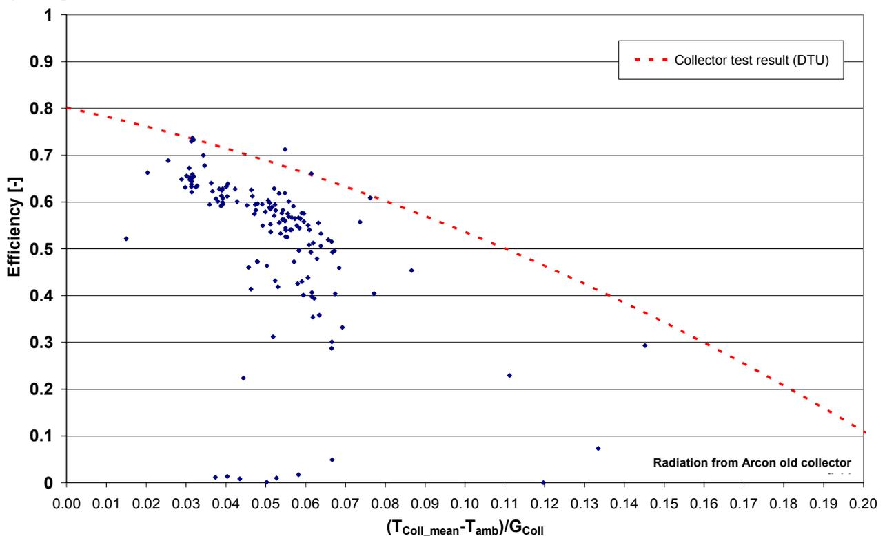
Fig. 2.26: Collector field efficiency Thermosol field (vacuum tube collectors, 108 m<sup>2</sup>)
