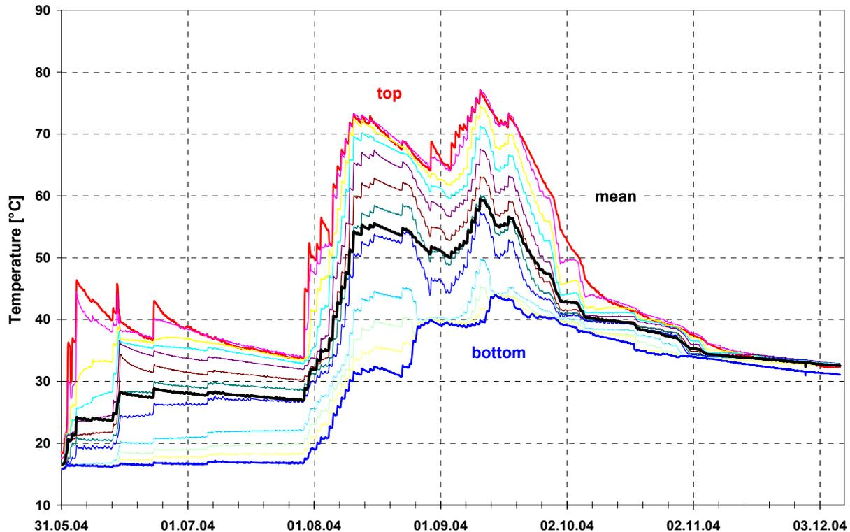
Fig. 2.30: Charging and discharging of the pit heat store
