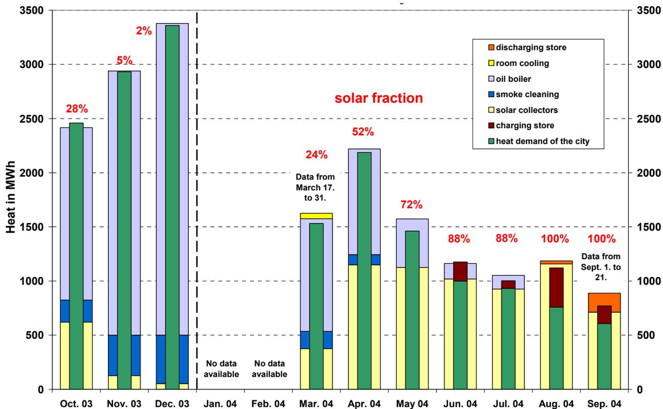
Fig. 2.18: System heat balance from October 2003 to September 2004 according to heat meter data
