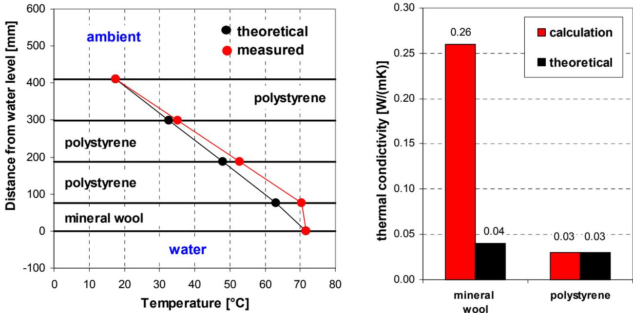
Fig. 2.33: Temperature gradient inside the cover construction (left) and theoretical and calculated thermal conductivities of the insulation materials (August 14<sup>th</sup> 2004)
