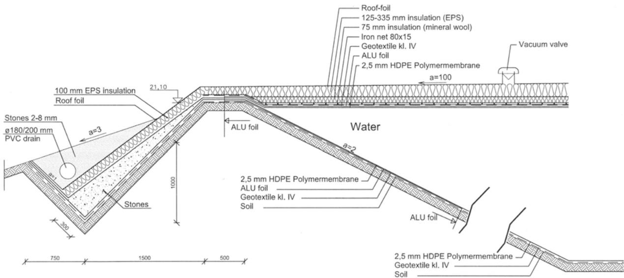
Fig. 2.10. Cross section of the edge of the pit storage.
