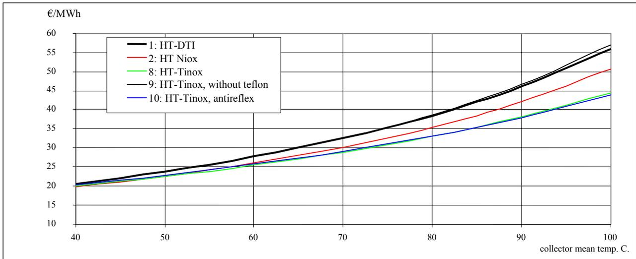
Fig. 2.4. Production price for heat for different collector combinations with Tinox absorbers.
