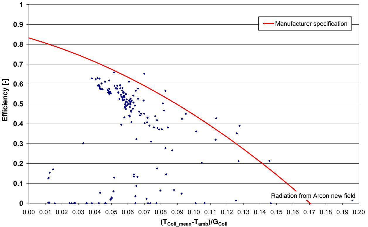
Fig. 2.25: Collector field efficiency Wagner field (103 m<sup>2</sup>)
