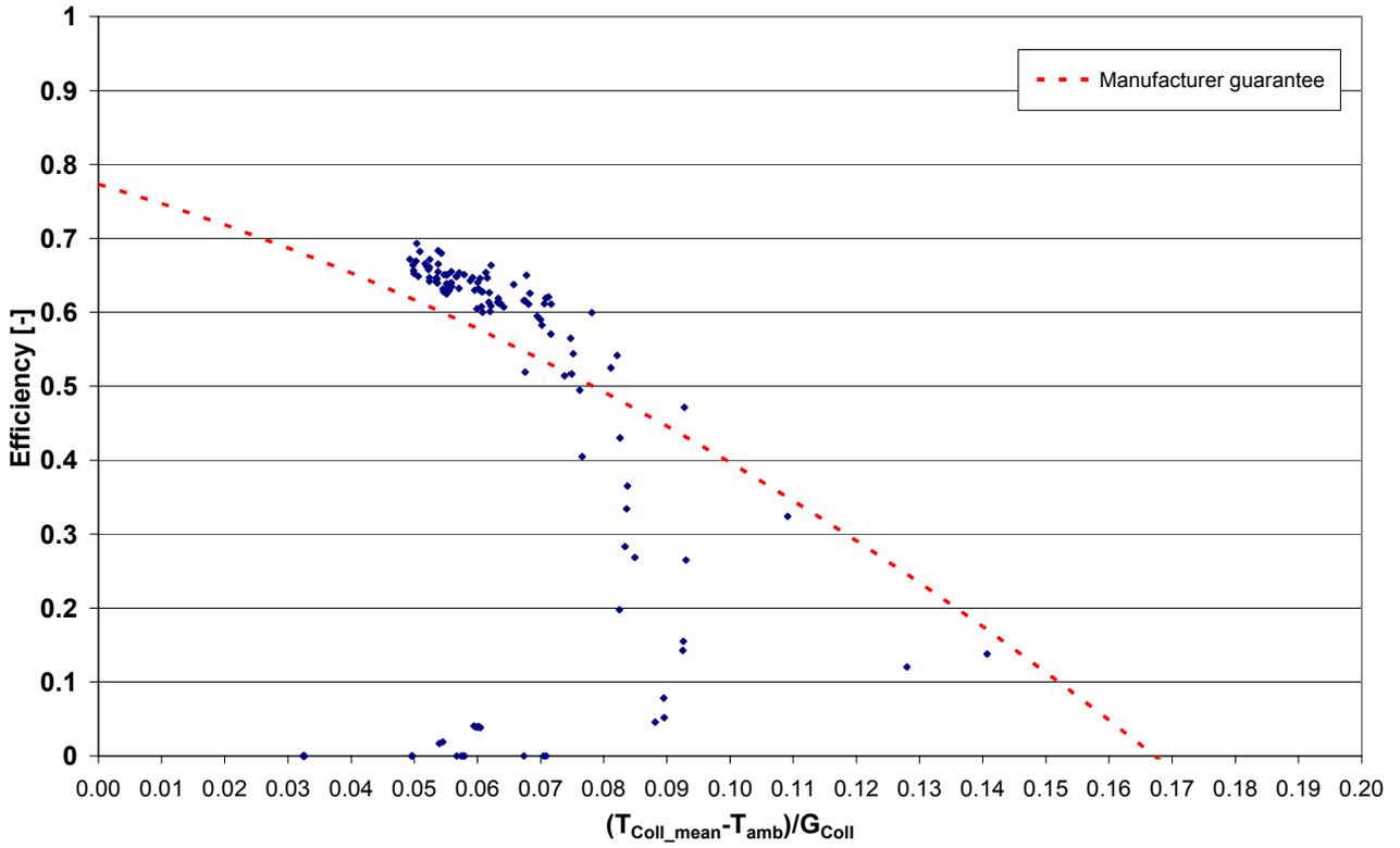
Fig. 2.24: Collector field efficiency GJ field (881 m<sup>2</sup>)
