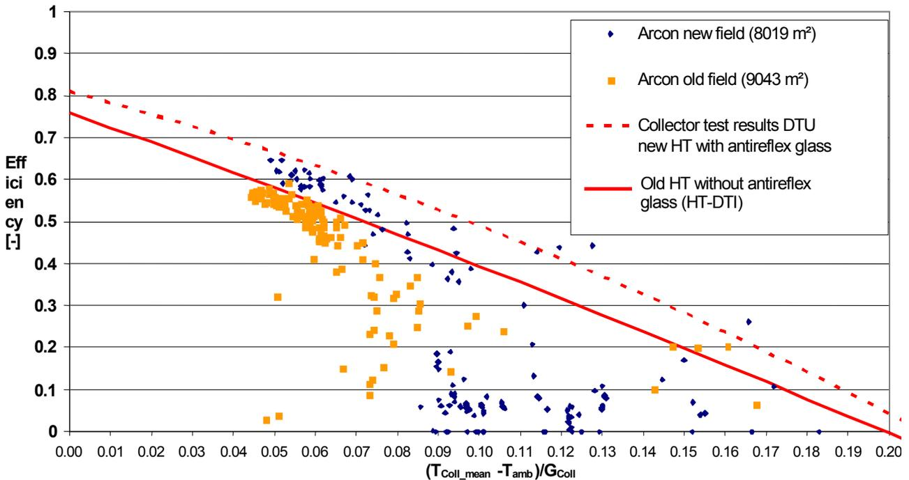
Fig. 2.23: Collector field efficiency Arcon collector fields
