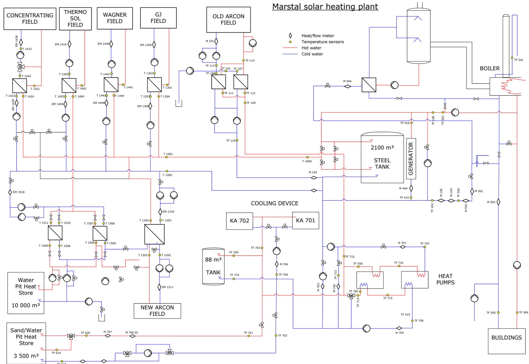
Fig. 2.16: Hydraulic plan of the Marstal solar heating plant with monitoring sensor positions
