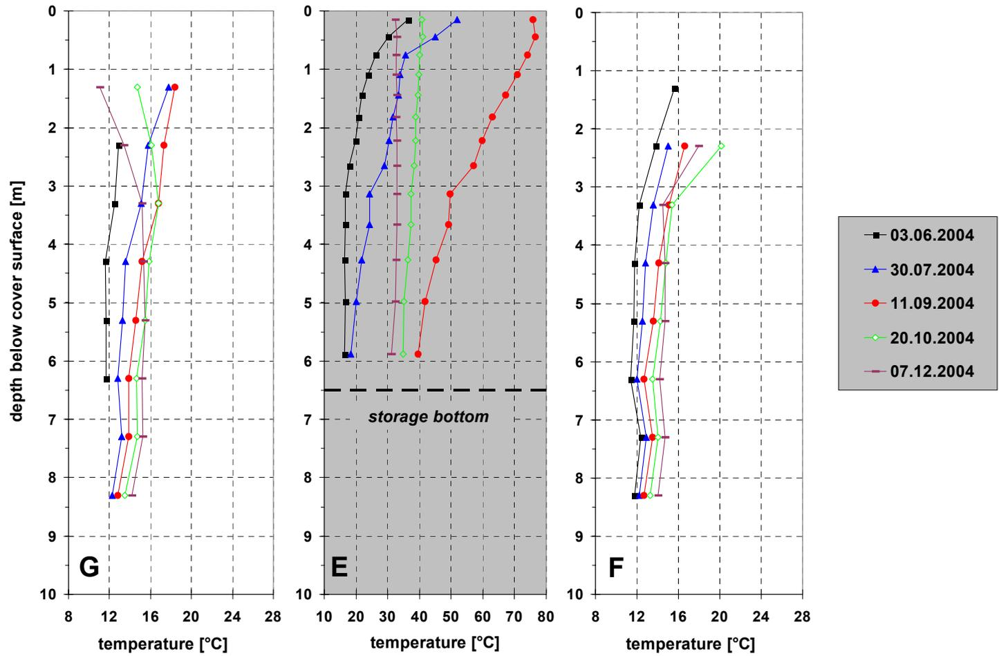
Fig. 2.32: Temperature development in and around the pit heat store (west – east direction)
