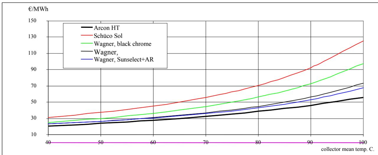
Fig. 2.7. Heat production prices from different roof modules.
