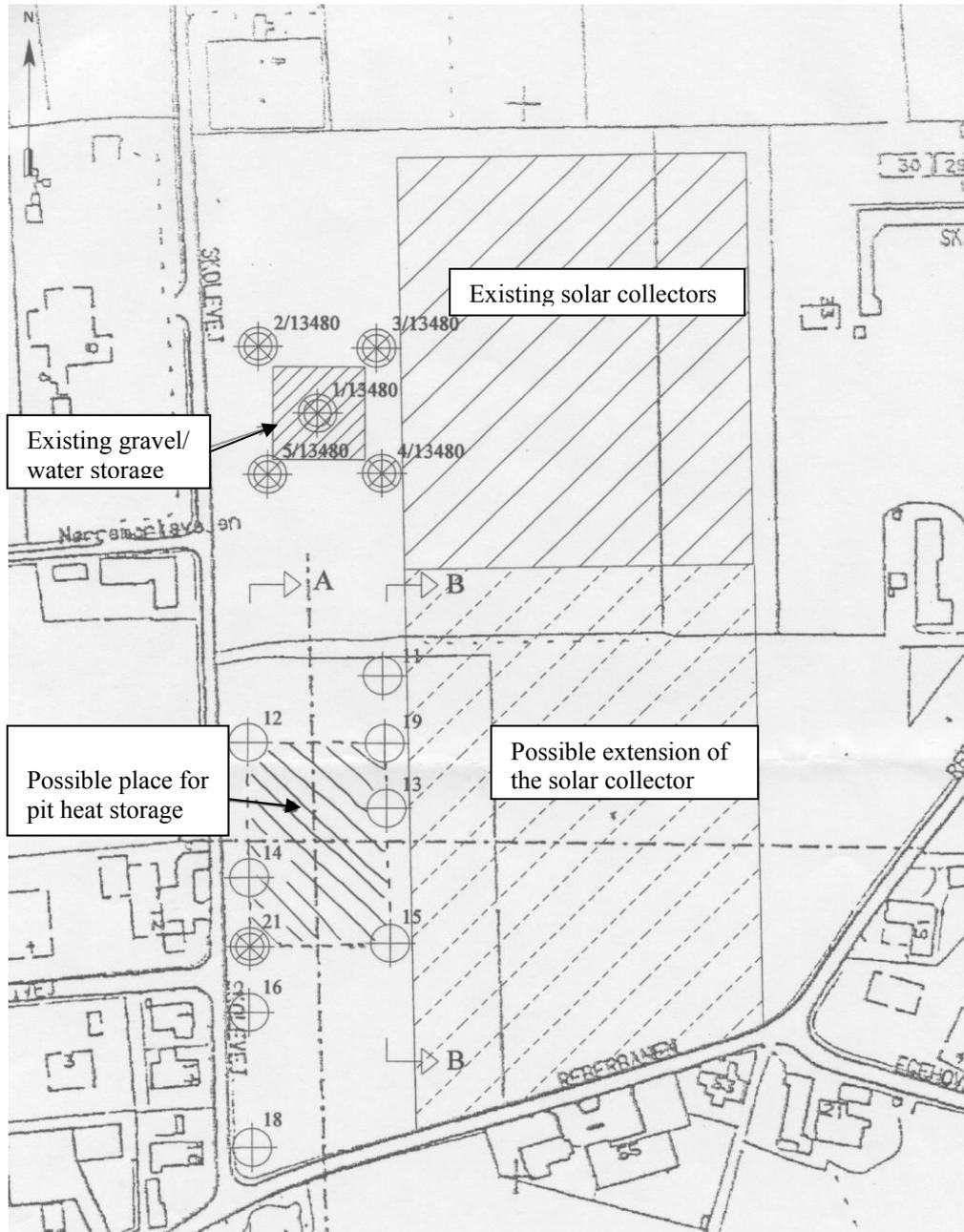
Fig. 2.1. Recommendation for position of pit heat storage.
