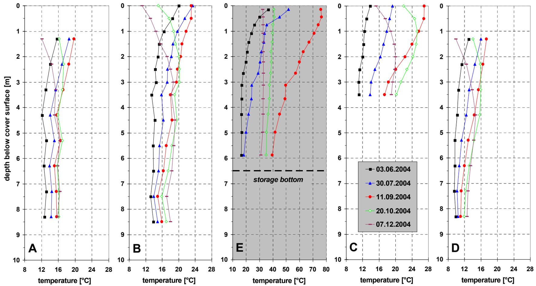
Fig. 2.31: Temperature development in and around the pit heat store (south – north direction)
